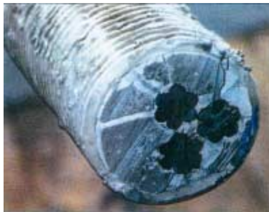
Photo 5: Strands encapsulated in grouted duct for free length protection.
